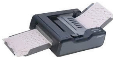
Fig. 2.15: OMR are used to read marks made using a pencil on a piece of pre-printed paper.
