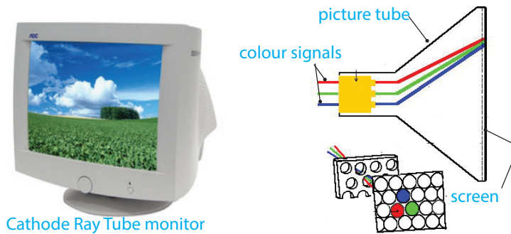
Fig. 2.32: The CRT monitor produces an image by firing electron beams.
