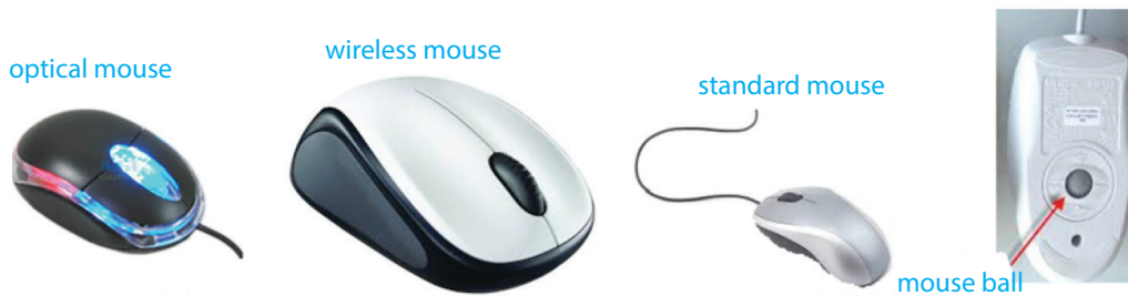
Fig. 2.8: A mouse is a pointing device with sensors that execute instructions by pointing.
