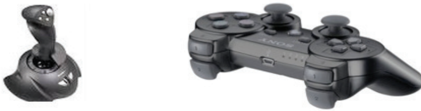
Fig. 2.10: A joystick looks like a gear lever. It is used to control the movement of the pointer.
