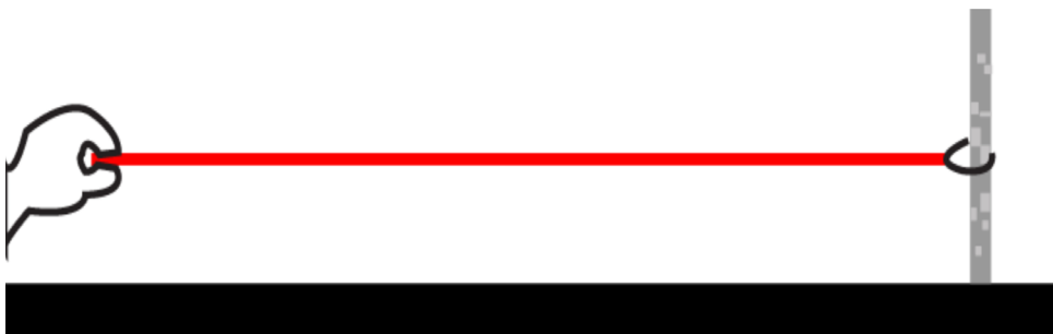
Fig.1. 5 An elastic rope that is not fastened to the pole used to study the behavior of a reflected wave at free end
