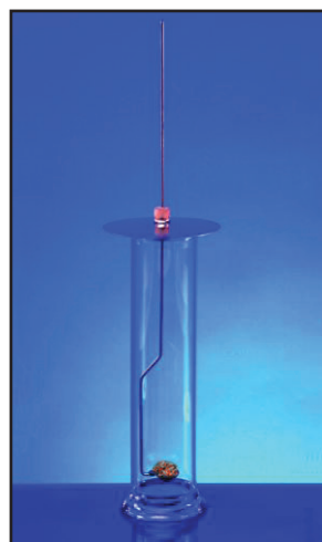
Fig 1.9 Burning charcoal in oxygen
