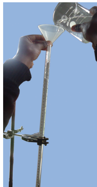
Fig 7.6: Correct method of filling a burette
