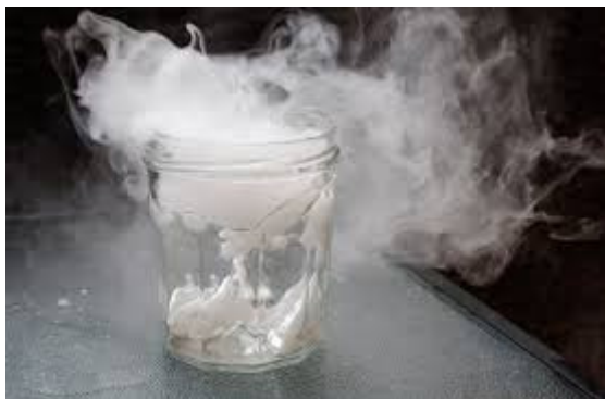
Figure 10.6. Sublimation of Dry ice at normal pressure
