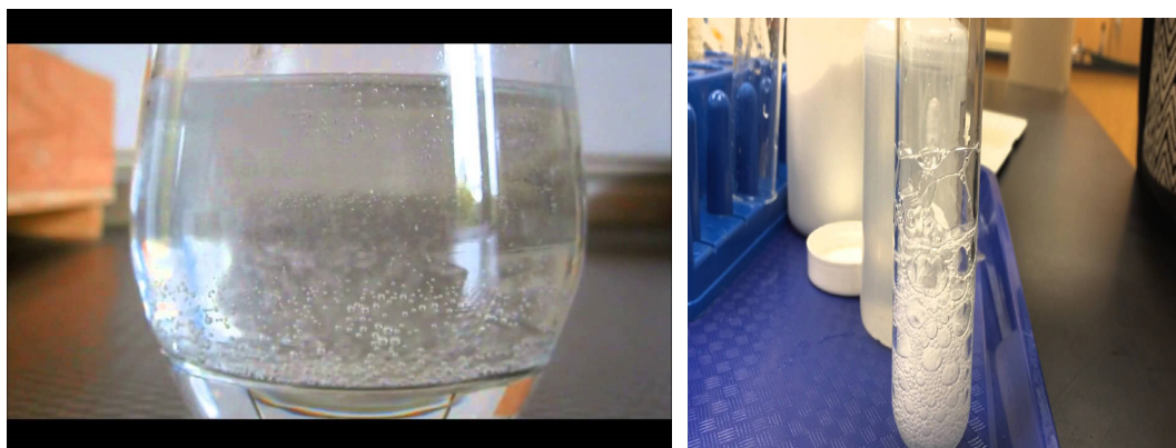
Figure 7.7. Effervescence when acetic acid is added to sodium carbonate
