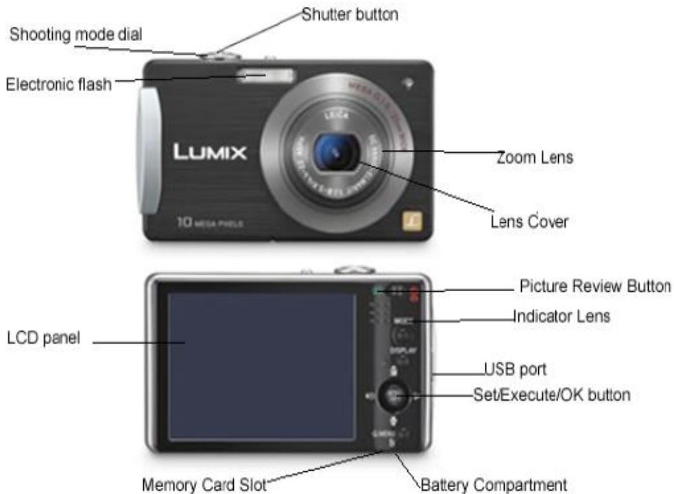
Figure 3. 6. Parts of a Digital camera
