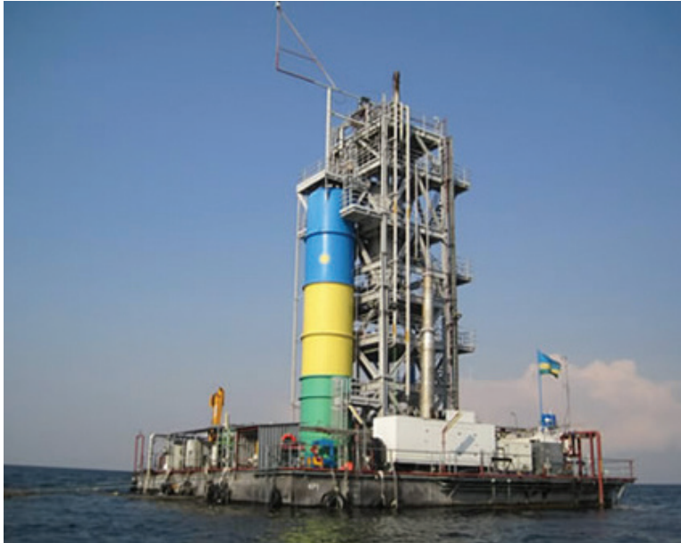
Figure 6.2: A methane gas extraction plant on Lake Kivu
