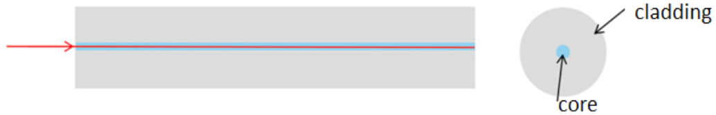
Fig.5. 8: Structure of monomode or single-mode optical fiber
