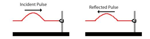
Fig.1. 6 Reflection of waves on a free end
