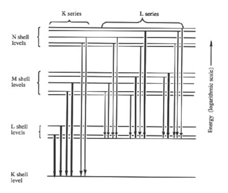
Fig.10. 1 Partial energy level diagram showing common transitions leading to X-radiation. The most intense lines are indicated by the widest arrows.
