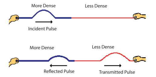
Fig.1. 10 A wave travelling from a more dense to a less dense medium will be reflected off the boundary and transmitted across the boundary into new medium. There is no inersion
