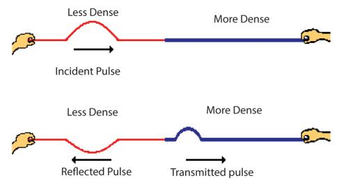
Fig.1. 8 A wave travelling from a less dense to a more dense medium will be reflected off the boundary and transmitted a cross the boundary into the new medium. The reflected pulse is inverted
