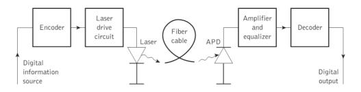
Fig.6. 3 A digital optical fiber link using a semiconductor laser source and an avalanche photodiode (APD) detector
