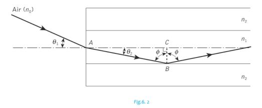
Assuming the entrance face at the fiber core to be normal to the axis, then considering the refraction at the air-core interface and using Snell's law given by  $n_0 \sin \theta_1 = n_1 \sin \theta_2$ .
