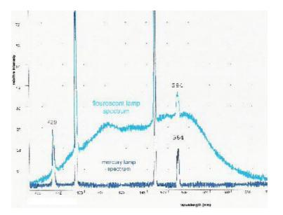
The fluorescent lamp's spectrum is a mixture of line and continuous spectra. Because of the exact correlation with the principal mercury vapor lines and the fluorescent lamp's lines, we can conclude that a major component of the fluorescent lamp is mercury vapor. But what produced the continuous portion of the fluorescent spectrum?
