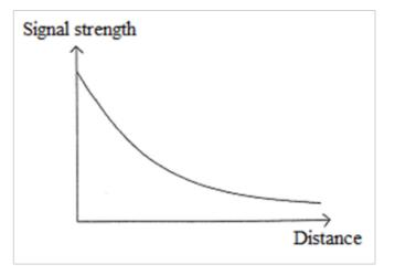
After 35 km, the signal strength is =  $0.95^{35} \times A = 0.166A$  (where A is the original signal strength).
