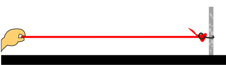
Fig.1.3 An elastic rope securely tied to a pole used to study the behavior of waves at a fixed end
