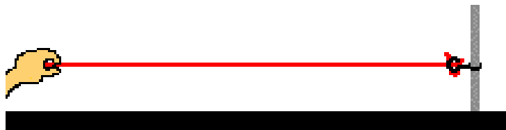
Fig.1. 14 An elastic securely tied to a pole can be used to study the behavior of waves at a fixed end
