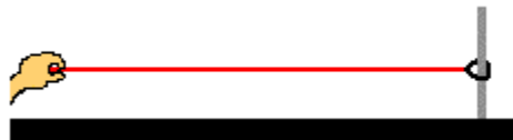
Fig.1. 16 If the end of elastic rope not fastened to the pole then it will be free to move up and down. This provides for the study of wave behavior at free end
