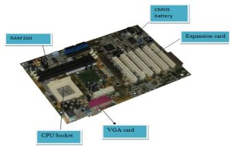
Figure 1.2 Motherboard and its different parts
