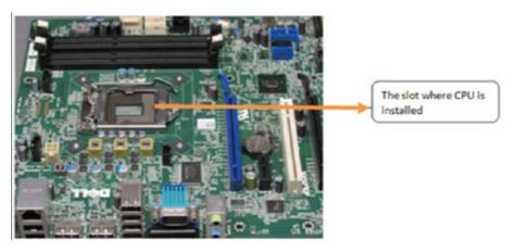
Figure 1.16 CPU Socket
