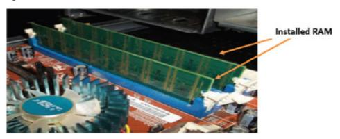
Figure 1.17 RAMs mounted on the motherboard
