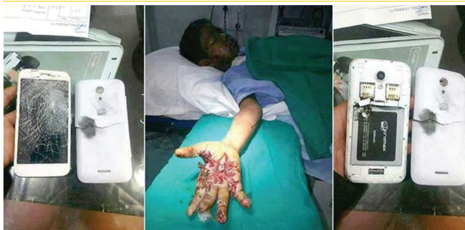
Figure 5.8: The phone burnt due to the high temperature developed in the battery during the charging and use of the phone at the same time
