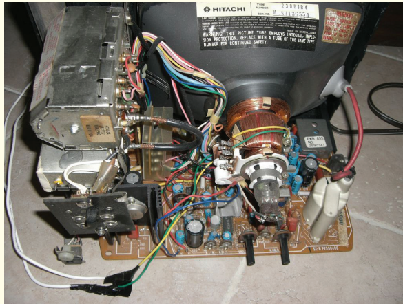
Figure 9.11: The inside of a TV set
