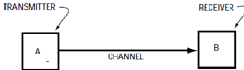
Fig.6. 1 Parts of communication system
