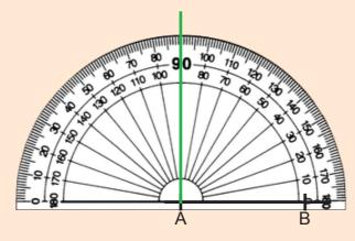
Step 3: From A, measure 3 cm along the 90° line. Label it D. Do the same at B and label it C.
