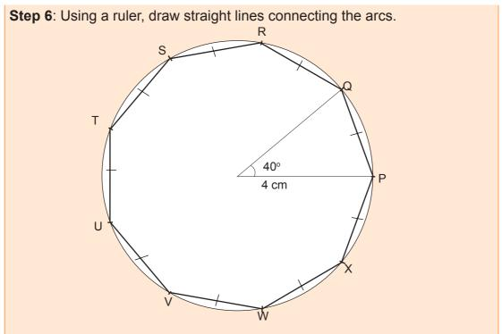
**Step 7**: Complete labelling the vertices. Mark sides with equal symbols. The regular polygon is a nonagon PQRSTUVWX.
