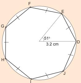
**Step 6**: Label the remaining vertices FGHIJ and the sides with equal signs. The figure is a regular septagon.
