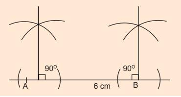
Step 3: Use a compass to measure and label points D and C from A and B of 4 cm respectively. Join D to C and name the rectangle ABCD.
