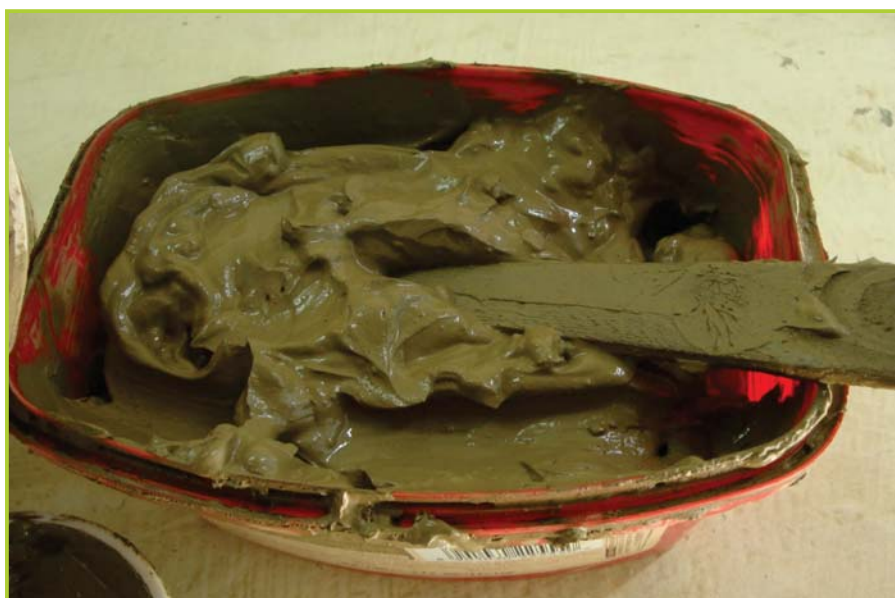
Figure 6: Slip ready to be used
