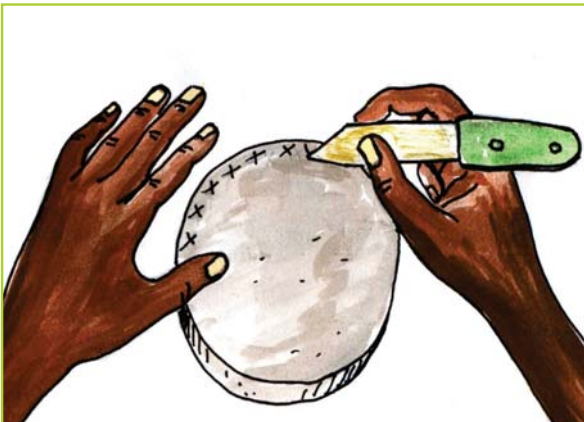
Figure 8: Scratching the slab with a knife
