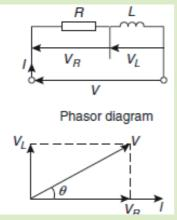
The analysis is similar but here, the p.d.  $V_L$  across Lleads on current I and the p.d.  $V_R$  across R is again in phase with I.
