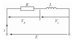
Figure 5.1. R-L series circuit
