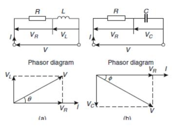
For example, in the **Resistance and Inductance** (R-L) series circuit shown in (a),  $V_L$  leads above figure, I by 90° (i.e. I lags  $V_L$  by 90°) and may be written as  $jV_L$ , the vertical axis being regarded as the imaginary axis of an
