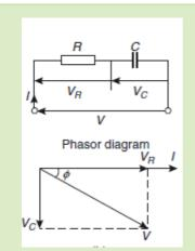
Vector sum of  $V_R$  and  $V_C$  is called **Impedance** and equals the applied p.d. V;
