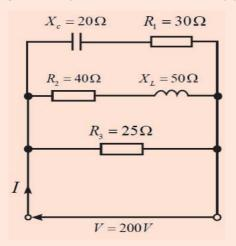
35. For the parallel circuit shown in the figure below, determine the value of current *I*, and its phase relative to the 240V supply, using complex numbers.
