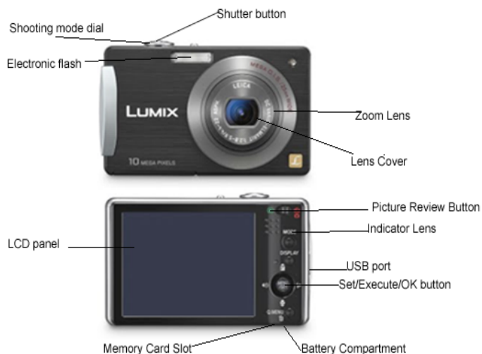
Figure 12.7 digital camera and its parts
