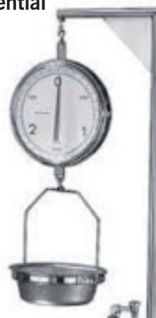
Fig. 9.3: Spring hang on retort stand
