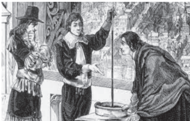
Fig. 4.6: Torricelli experiment of a simple mercury barometer
