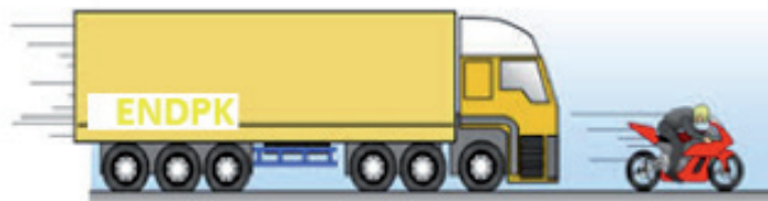
Fig. 8.4: The Kinetic energy of a moving body depends on its mass and velocity
