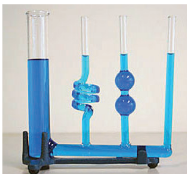
Fig. 5.10: Communicating vessels or Pascal's vessel
