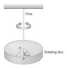
Fig.2-1; Torsional pendulum
