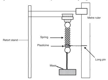
Fig.2-4; Oscillation of a mass on spring
