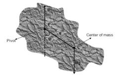
Fig.2-2; Compound pendulum
