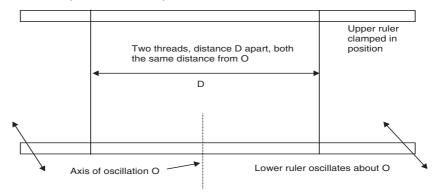
Fig.2-3; Bifilar suspension
