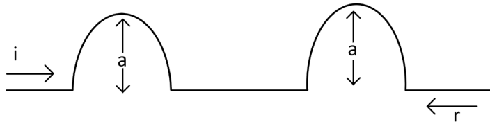
Fig.4. 7 progressive waves of the same amplitude and frequency, travelling in opposite directions.
