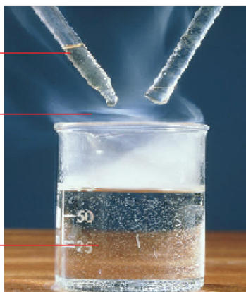
Figure 13.6.a. Reaction of ethanoyl chloride with water produces white fumes
