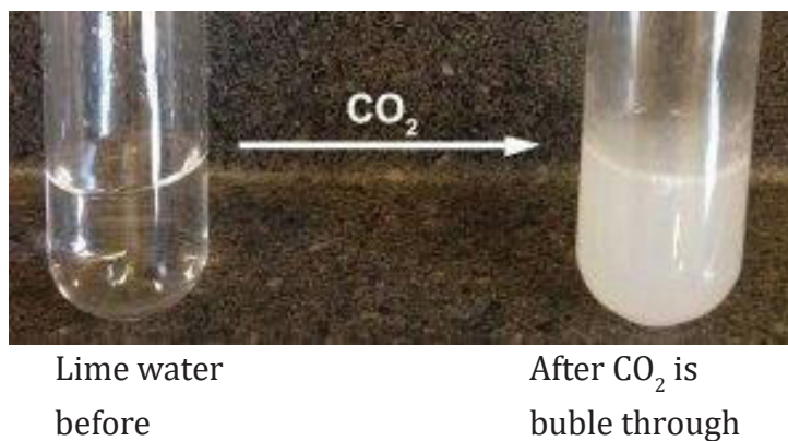
Figure 13.7. Testing carbon dioxide by lime water
