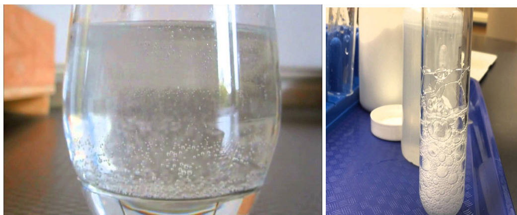
Figure 13.6. Effervescence when acetic acid is added to sodium carbonate
