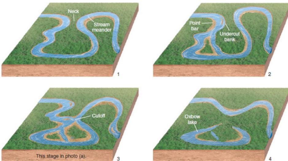
*Development of a river meander and an oxbow lake simplified in four stages*
