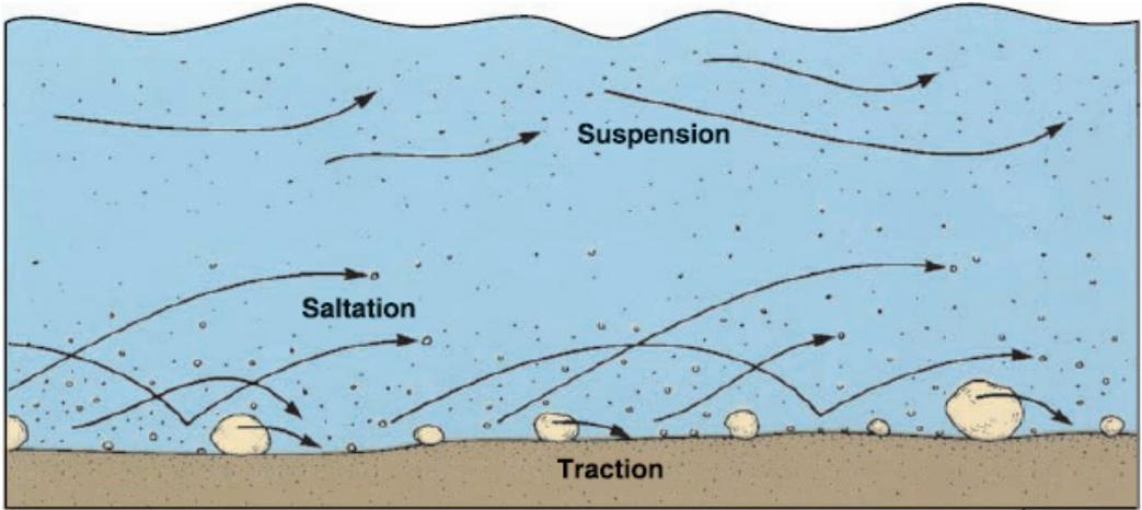
**Transport of solid load in a stream:** Clay and silt particles are carried in **suspension**. Sand typically travels by **suspension** and **saltation**. The largest (heaviest) particles move by **traction**.
