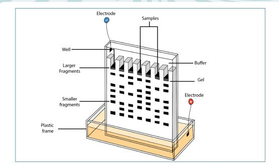
Figure 4.5: Fragments arrangement in gel electrophoresis
