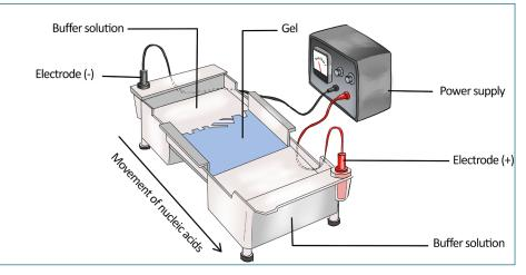
Figure 4.3: Setup of gel electrophoresis
