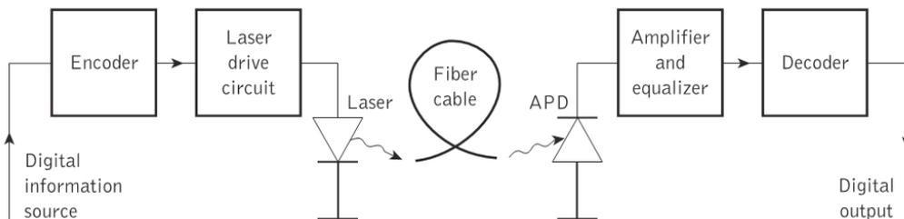
Fig. 6. 1 A digital optical fiber link using a semiconductor laser source and an avalanche photodiode (APD) detector
