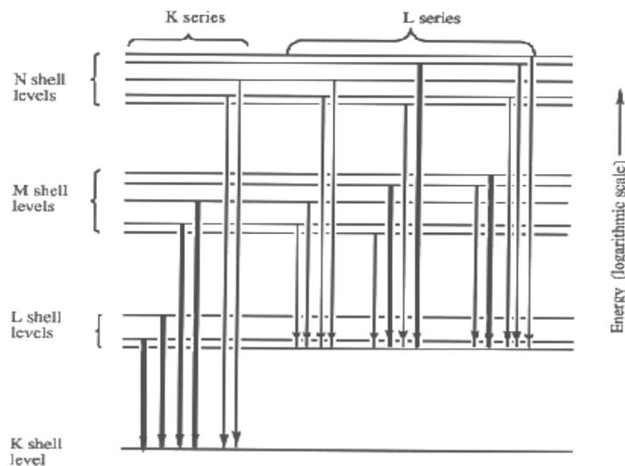
Fig.5. 1 Partial energy level diagram showing common transitions leading to X-radiation. The most intense lines are indicated by the widest arrows.
