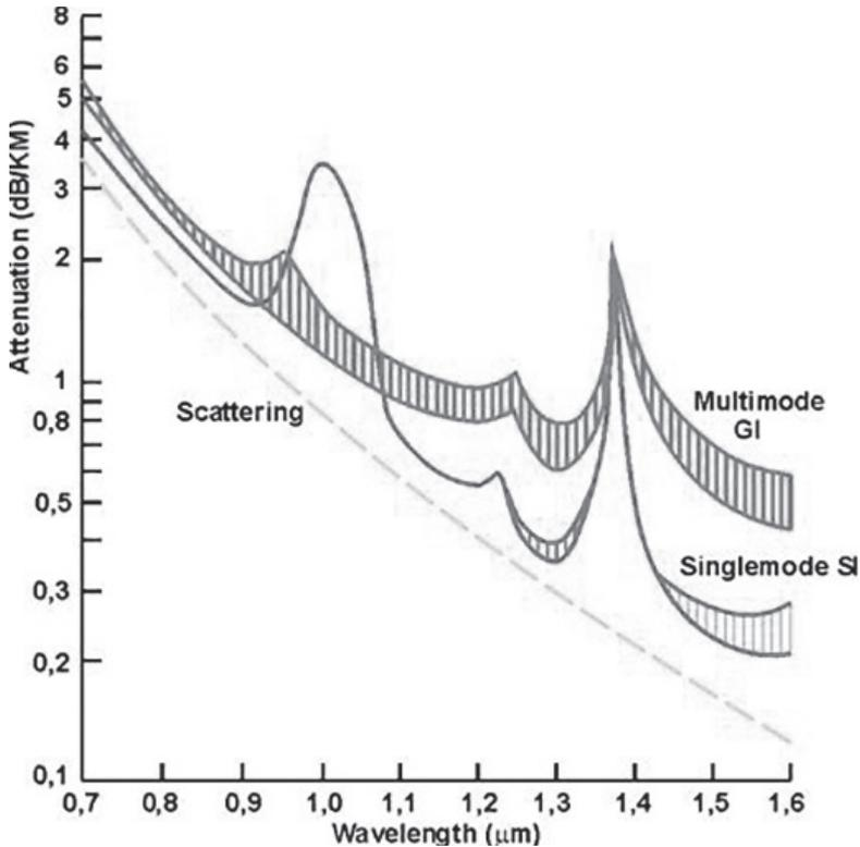
Fig.3. 3 Attenuation of the single mode step index (SM SI) and multimode graded index (MM GI) silica glass fibers as a function of a wavelength.
