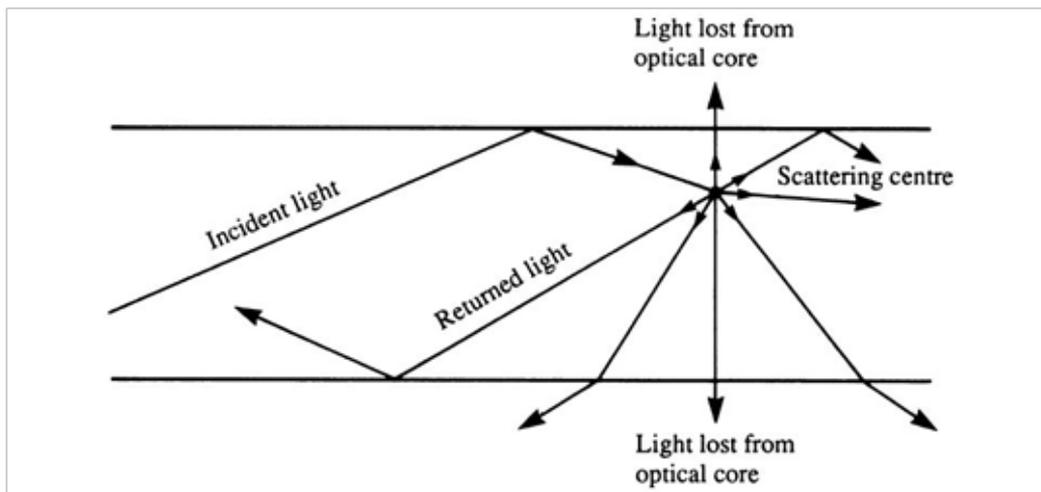
Fig.3. 1: Light scattering in optical fiber
