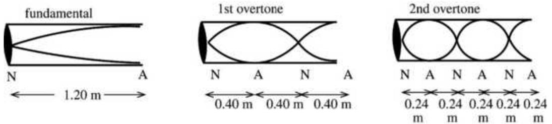
Fig.1. 3 Standing waves produced by pipe open at one end and closed at the other end
