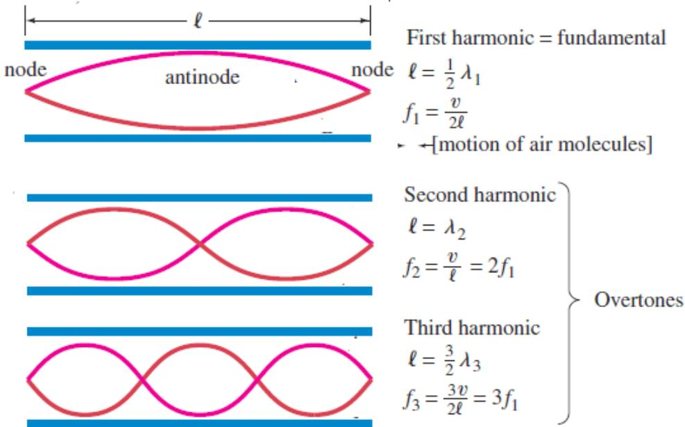
Fig.1. 1 Pressure variation in the air: Graphs of the three simplest modes of vibration (standing waves) for a uniform tube open at both ends ("open tube").
