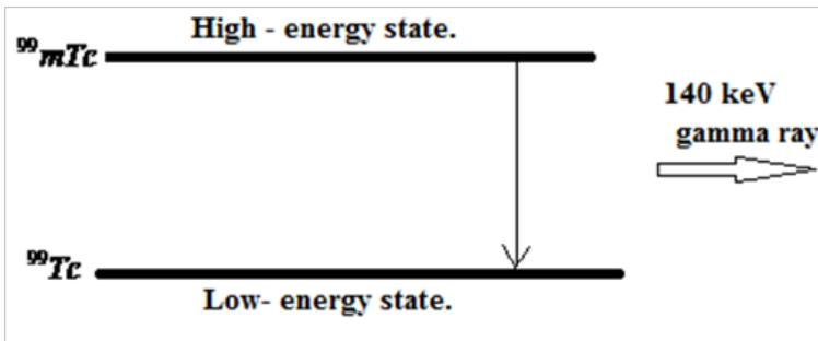
Fig7.12: Gamma ray production. The metastable atom  $^{99m}\text{Tc}$  passes from a high-energy to a low-energy state and releases gamma radiation with a peak energy of 140 keV.
