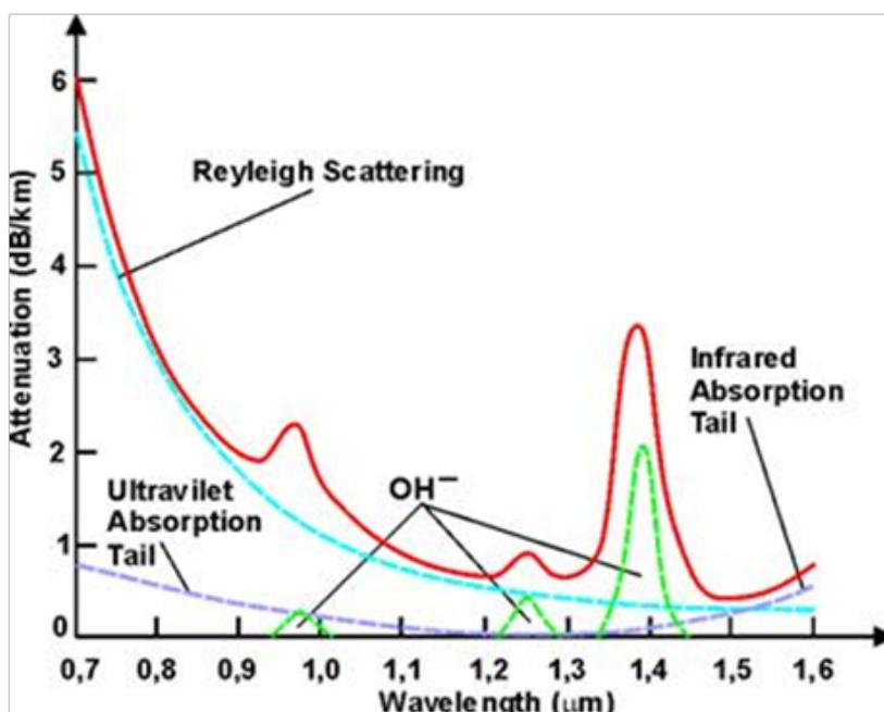
Fig.3. 2 Spectral attenuation of a silica optical fiber
