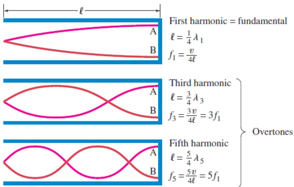
Fig.1. 2 Modes of vibration (standing waves) for a tube closed at one end ("closed tube")
