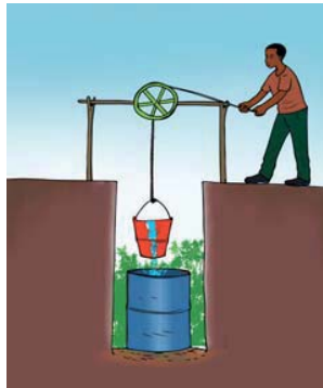
Fig 2.6 Windlass is an example of wheel and axle
