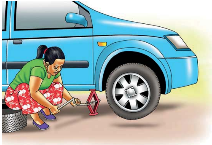
Fig 2.10 Screw jack in use
