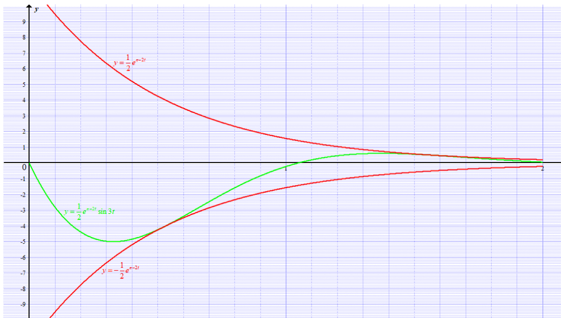
Figure 4.13: comparison of the graph of y = \frac{1}{2}e^{-2t} , y = \frac{1}{2}e^{-2t} \sin 3x and y = -\frac{1}{2}e^{-2t} Hyperphysics..phy-astr.gsu.edu/hbase/osca2.html .
