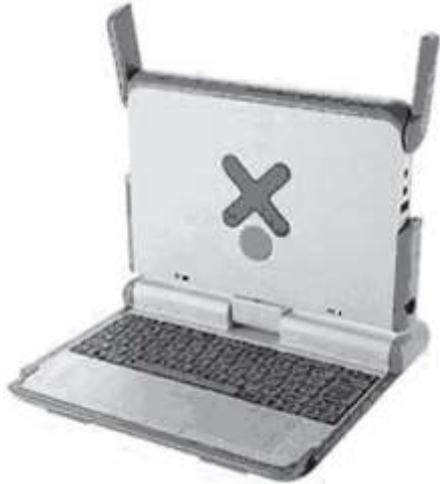
3. Lay the display down onto the keyboard.
