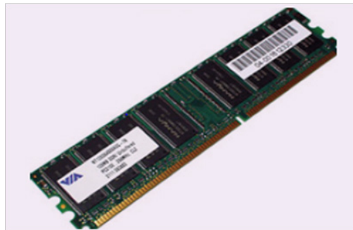
Figure 2. 6. An example of a Random Access Memory
