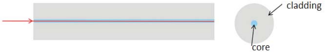
Fig.6. 8: Structure of monomode or single-mode optical fiber
