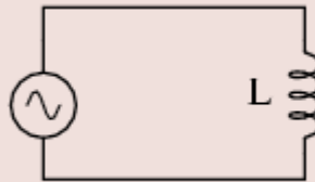
Fig. 11.24: An inductor connected to an a.c supply
