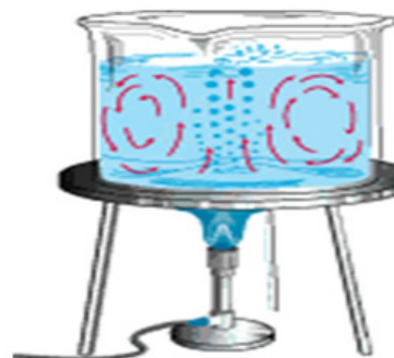
Fig. 15.2: convective currents in water
