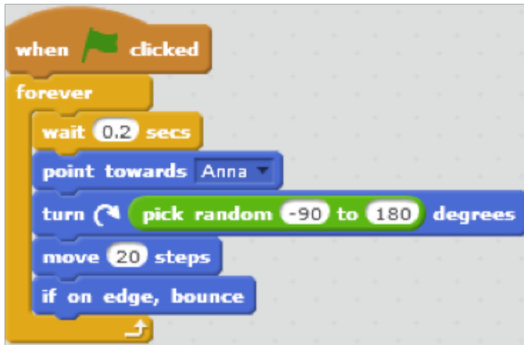
Figure 9.34: Motion script to fly the Bat towards Anna with some randomness and in all four directions
