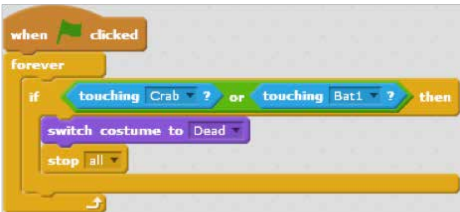
Figure 9.35: Script that would make Anna to die when touched by the Crab or Bat
