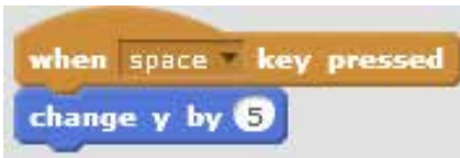
Figure 9.39: Script to control the up of the helicopter
