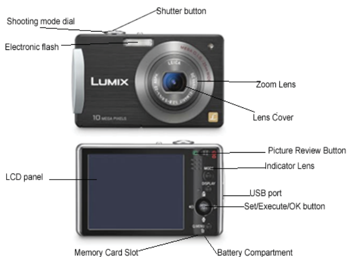
Figure 12.7 digital camera and its parts
