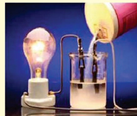
Sodium chloride solution, \text{NaCl}(aq) electrolyte conducts electricity
