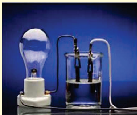
Pure water, \text{H}_2\text{O}(l) does not conduct electricity
