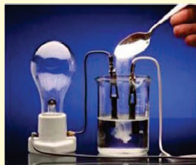
Sucrose solution, \text{C}_{12}\text{H}_{22}\text{O}_{11}(aq) non-electrolyte does not conduct electricity
