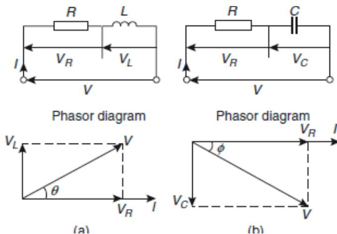
For example, in the **Resistance and Inductance** ( $R-L$ ) series circuit shown in (a),  $V_L$  leads above figure,  $I$  by  $90^\circ$  (i.e.  $I$  lags  $V_L$  by  $90^\circ$ ) and may be written as  $jV_L$ , the vertical axis being regarded as the imaginary axis of an
