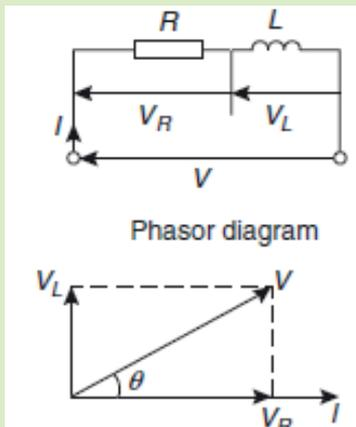
Figure showing Resistance and Inductance in series
