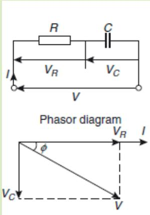
Figure showing Resistance and Capacitance in series
