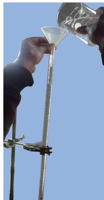
Fig 7.6: Correct method of filling a burette
