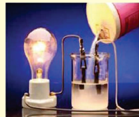
Sodium chloride solution, \text{NaCl}(aq) electrolyte conducts electricity
