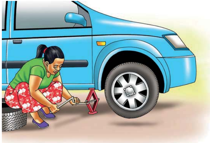
Fig 2.10 Screw jack in use
