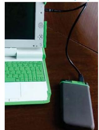
Fig. 4.8: External hard disk connected to an XO laptop.
