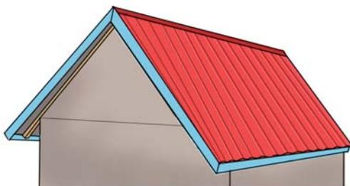
Fig. 16.4: Painted iron sheet roof.
