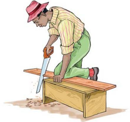
Fig. 1.3: Using a wood saw.
