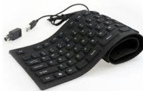
Fig. 2.5: A flexible keyboard can easily be folded and carried in a bag.
