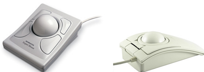
Fig. 2.9: A track ball is a pointing device with a ball on the top that is rotated with the finger.
