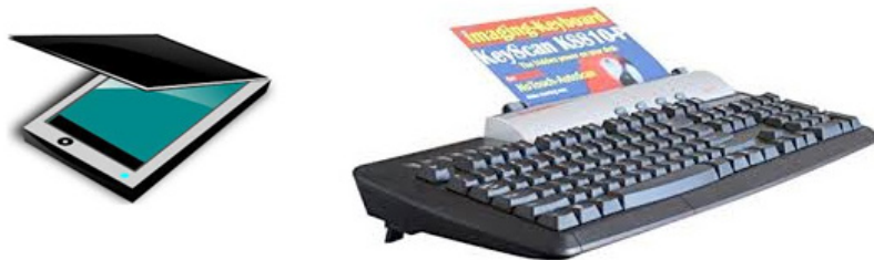
Fig. 2.16: OCR is used for reading hardcopy data into a softcopy that is stored in the computer.
