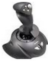
Fig. 2.10: A joystick looks like a gear lever. It is used to control the movement of the pointer.
