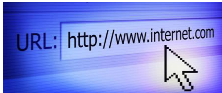
Fig. 8.6: The URL consists of the protocol, the server name and the resource ID.
