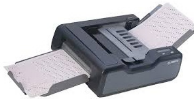
Fig. 2.15: OMR are used to read marks made using a pencil on a piece of pre-printed paper.
