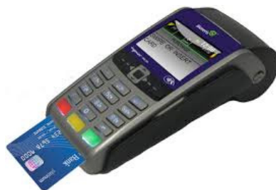
Fig. 2.18: A Mobile Card Machine reads data contained in a chip embedded in plastic cards.
