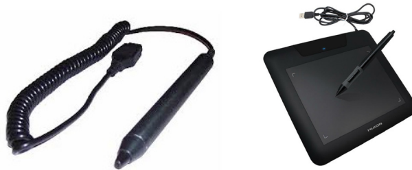
Fig. 2.11: A light pen is an input device that utilizes a light sensitive detector to select objects.
