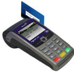
Fig. 2.19: The Magnetic Stripe Card Reader
