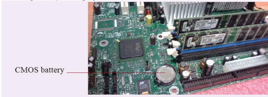
Figure 1.9. CMOS battery
