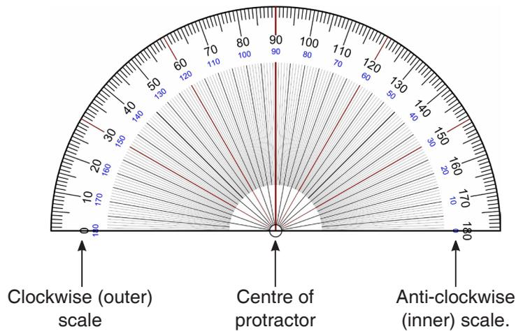
The above protractor can be used to measure angles from  $0^\circ$  up to  $180^\circ$ . Angles can be measured either in a clockwise sense or anti-clockwise sense depending on where the angle is drawn.
