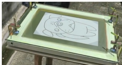
Figure 3.11: sticking a design on screen print
